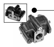
The design of this unit takes advantage of relatively low pressure operating requirements (450 psi.) to reduce the number of cast iron components required for its two pump sections from five pieces to three. Relief valves for both sections are built into the pump body. The common journal carrier, one-piece steel drive shaft, and powdered metal driven gears contribute to the overall compactness of the design while providing charge and transmission lubrication flows.
