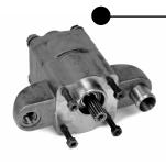
This unusually-shaped shaft end housing allows it to fit tight mounting spaces while maintaining smooth hydraulic line functions. The housing features integral port lobes that allow straight hydraulic line connections without line kinks or space robbing line loops. Overall length of the pump is reduced by eliminating typical gear housing ports.
