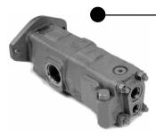
By incorporating the priority flow valve and relief valve in the port end housing, this design puts the added flow of a tandem to good use without requiring excessive mounting space for a bolt-on valve. The integral priority flow valve provides primary and secondary flow ports. Flow in excess of that required by the priority circuit may be routed to a power beyond function. These units may be used to provide power steering or braking requirements.
